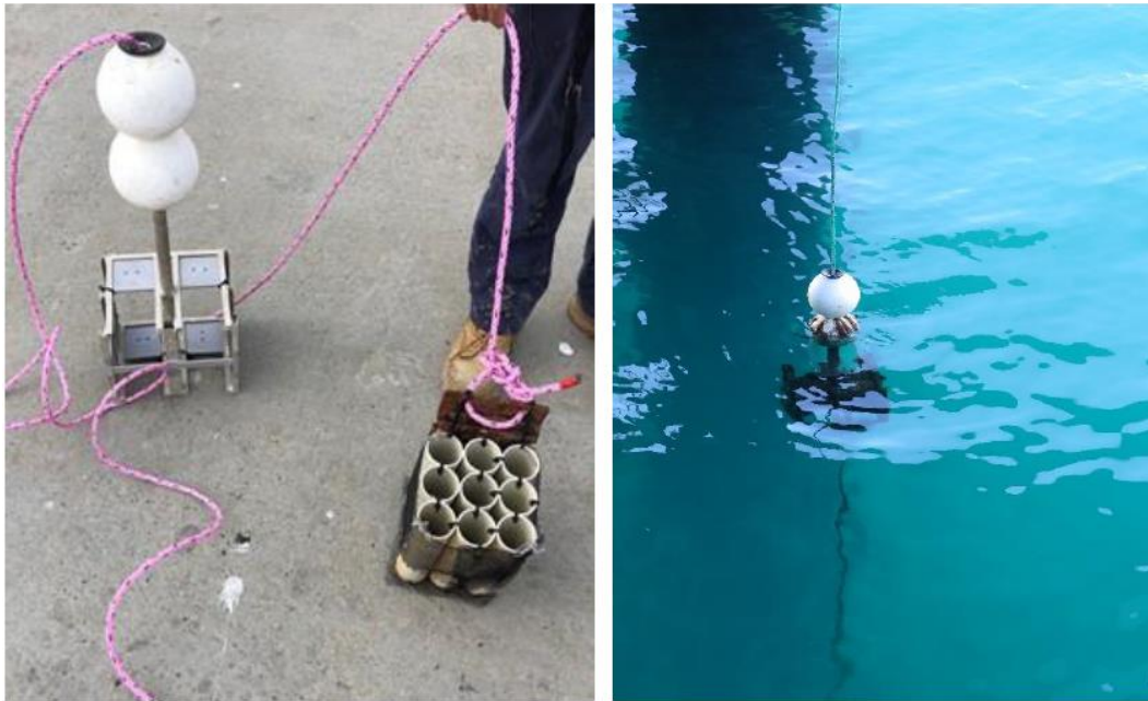
Photo 24 Box array and crab condo ready for deployment (left) and box array deployed in-water (right)
