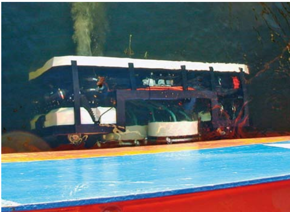
Figure 3.5 CleanROV, an automated hull cleaning vehicle
