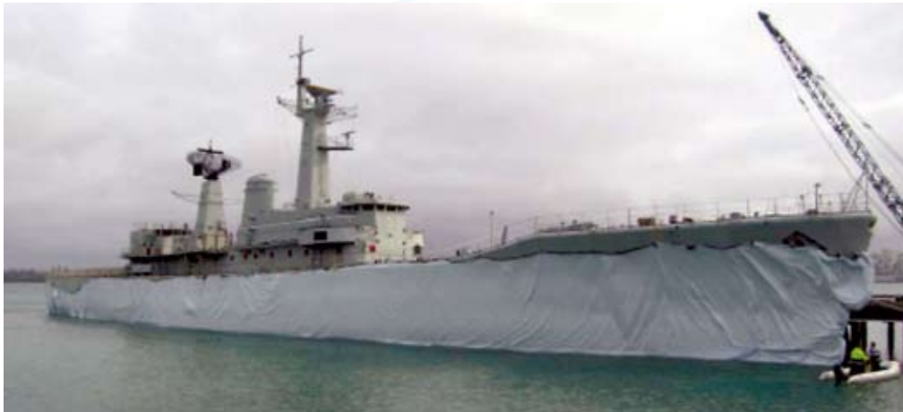
Figure 3.11 The New Zealand naval frigate Canterbury encapsulated in plastic
