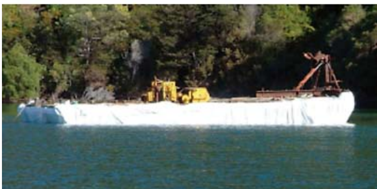
Figure 3.10 Encapsulation of recreational and commercial vessels of 7–30 m in length in the Marlborough Sounds, New Zealand
