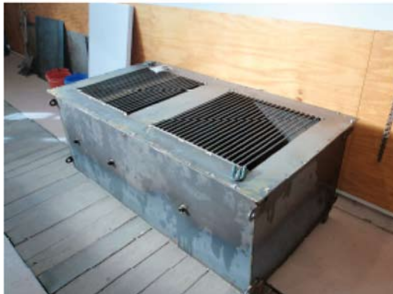
Figure 3.9 The sea chest sterilisation model developed by the University of Canterbury
